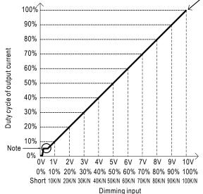
100% when DIM+/DIM- are open circuit.
