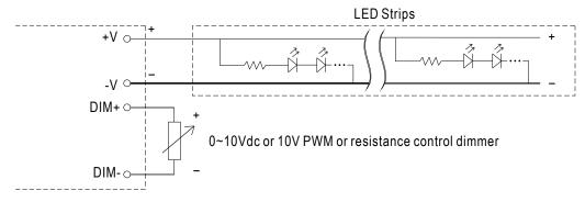
"DO NOT connect "DIM- to -V"
